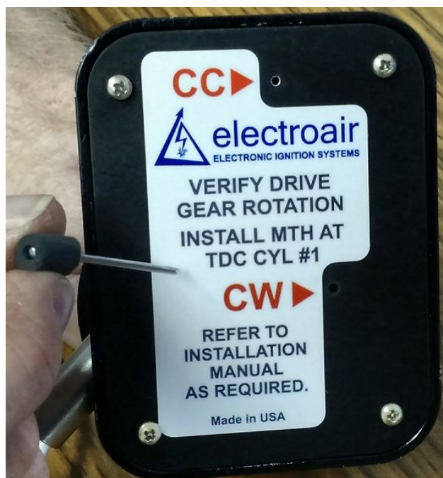
Figure 7: Installation of MTH Alignment Pin
