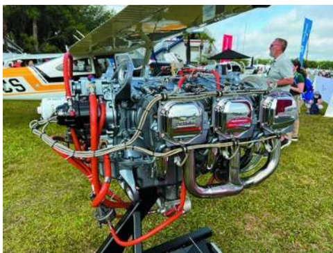
This is the TIO-40-AK1A, for the in-certification Cessna T182T turbo Skylane, which is on Electroair's AML-STC
