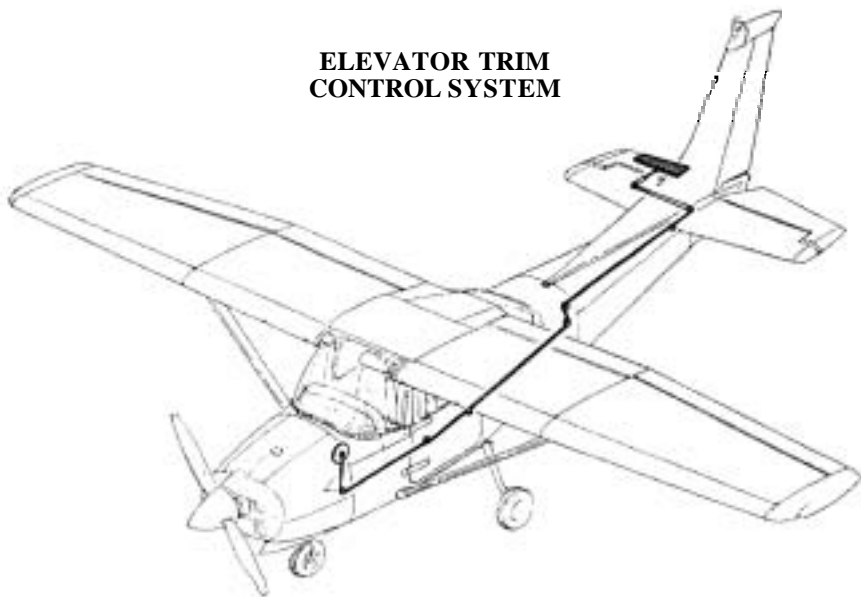
Figure 7-1. Flight Control and Trim Systems (Sheet 2 of 2)
