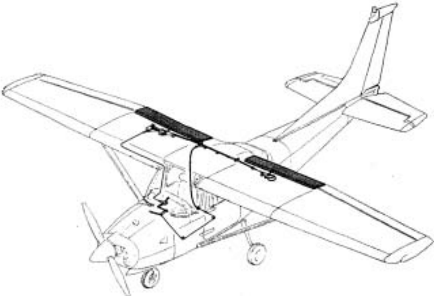
Figure 7-3. Wing Flap System
