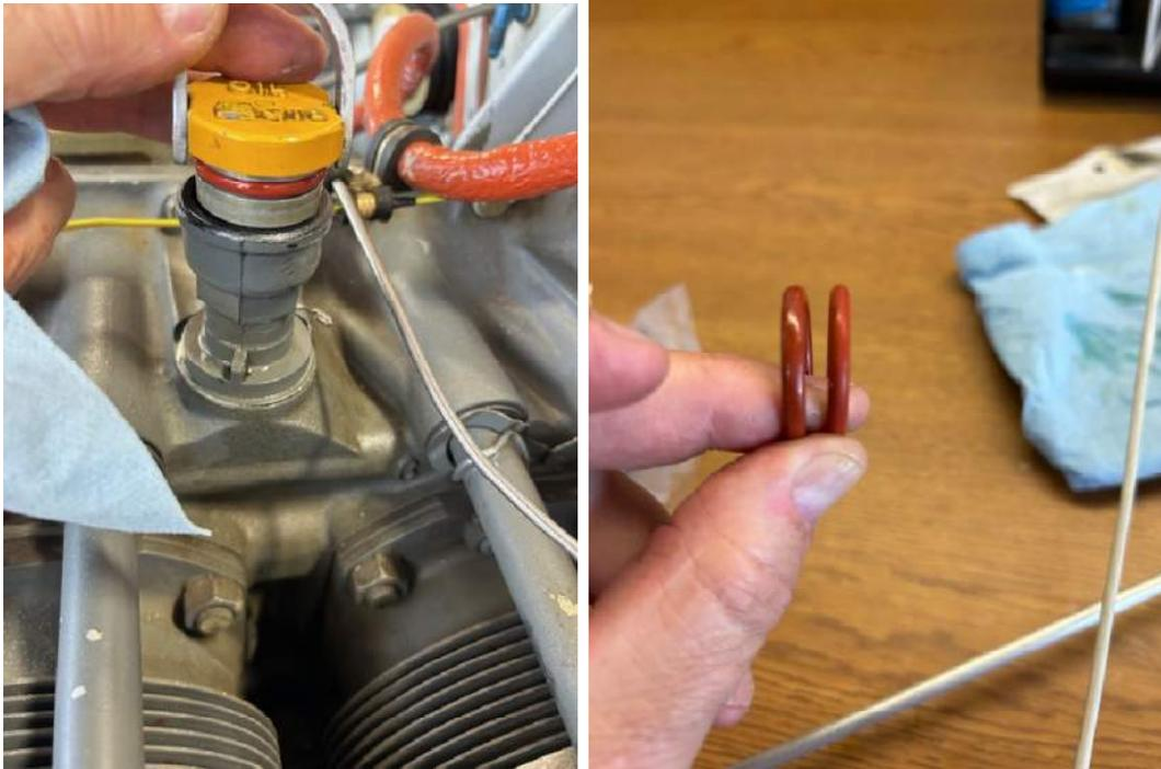
Removal of the old o ring is easy but take care not to score the dipstick. The filler base is drier than previous and the dipstick has noticeably more friction(requires 2 hands) to install, compared to it falling into place past the détente with the old o ring.
