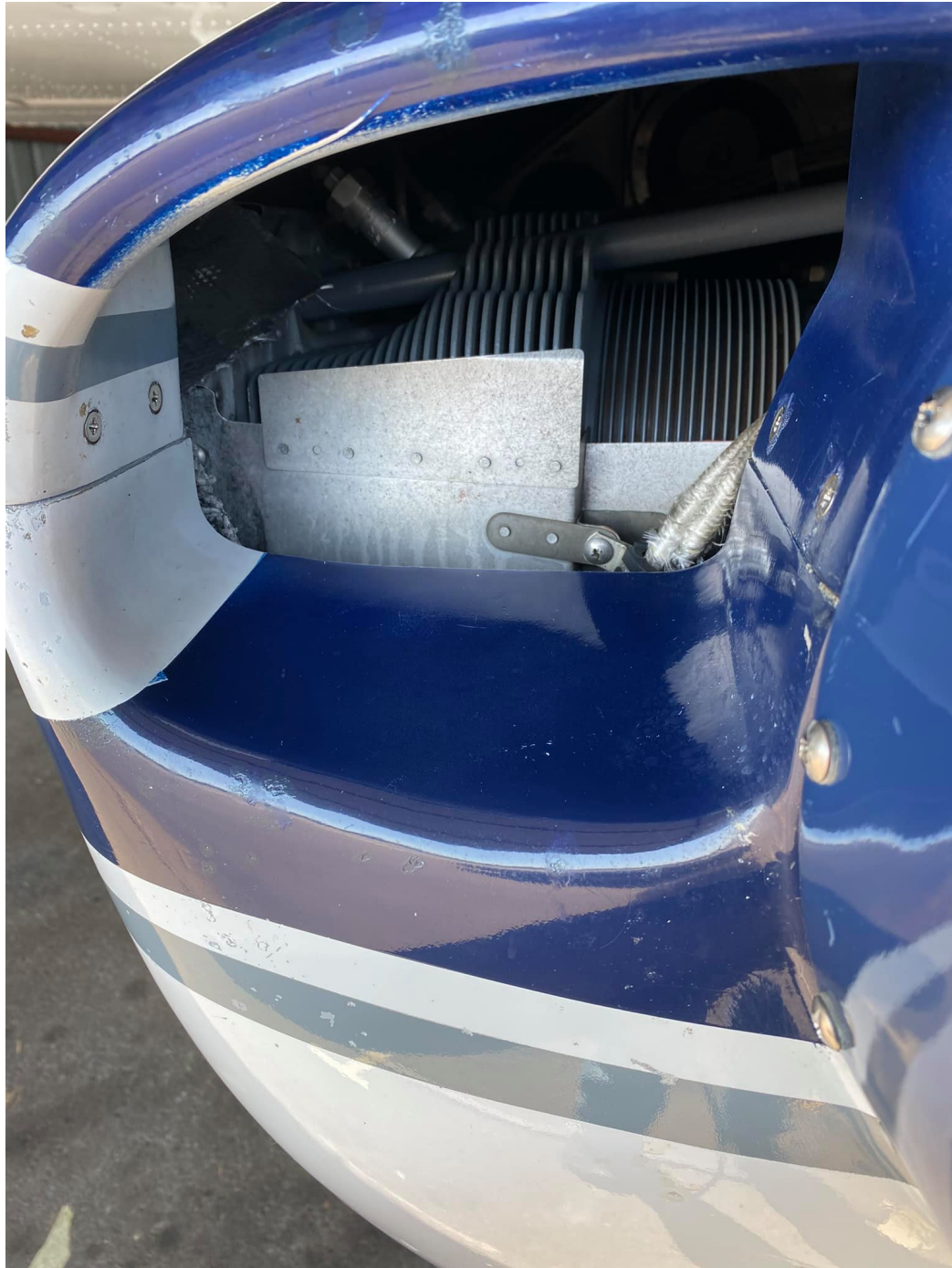
High version of baffle in front of cylinder 1
