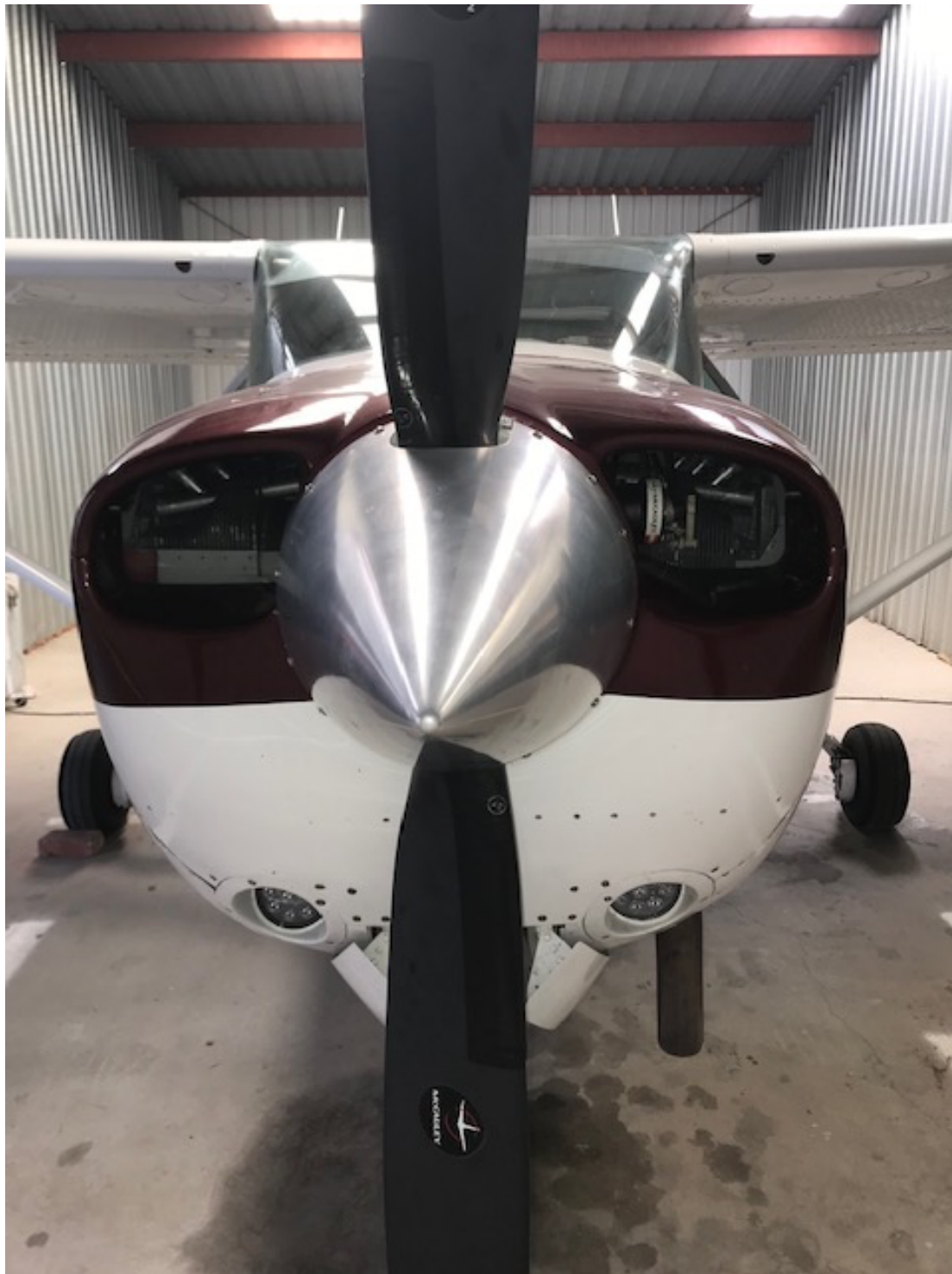
Top part of baffle removed in front of cylinder 1
