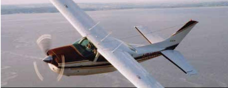
*Micro VGs are installed on the leading edge of the wings and on tail surfaces to help keep air attached longer at slower speeds. This reduces the Stall Speed, improves controllability, improves characteristics, creates a more stable instrument platform and gives better aileron response and rudder authority without reducing cruise speed.*
