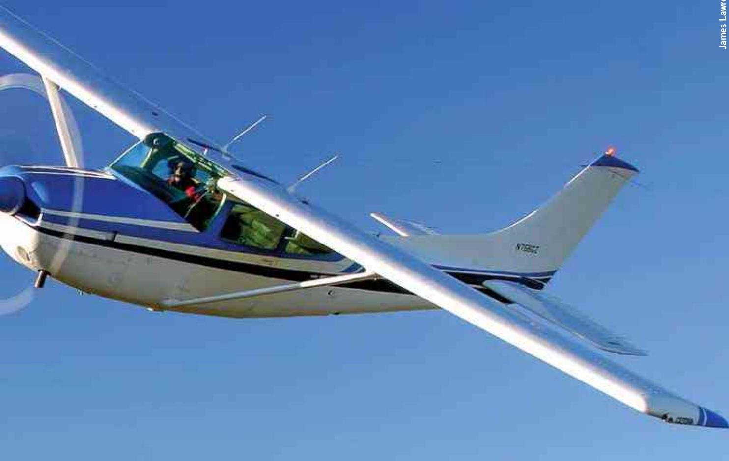
you need a turbo to operate in the mountains? No, but your operating limitations will increase without one. While both the turbo and non-turbo aircraft feel the same air molecules flowing over the wing, the engine experiences entirely different induction airflow mass, and the turbo will make significantly more power. You *will* notice the difference.
