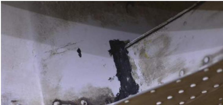
Forward end of wheel well after sealant application.
