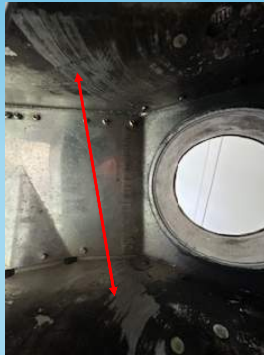
Membrane marks on airbox walls
