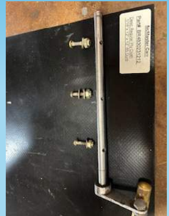
Butterfly pivot arm attachment in good condition
